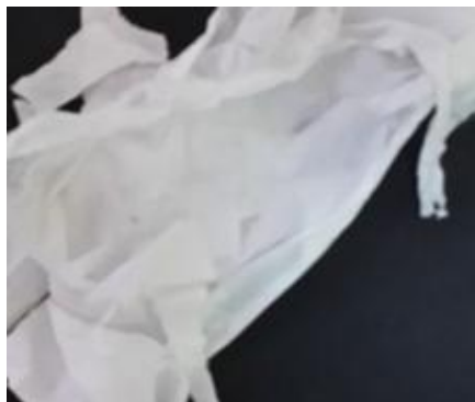
Figure 4. a photo of electrospun acrylic sample
