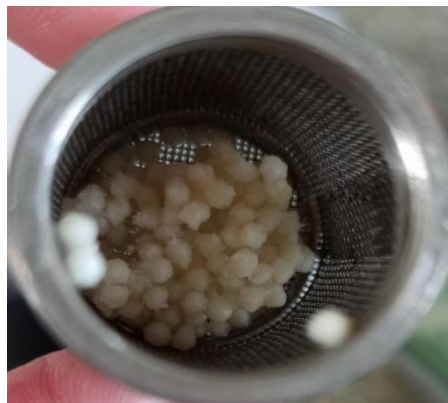
Fig. 5: swelling of metformin HCl- loaded alginate beads in phosphate buffer.
