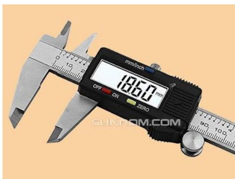
Figure 2 shows the digital Vernier caliper used for measurements.
