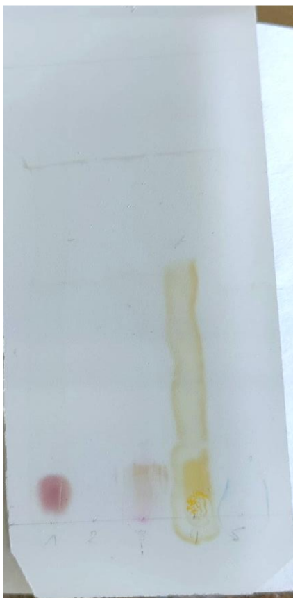
Figure 4: Qualitative Analysis of Metals Using Merck Paper for Chromatograms
